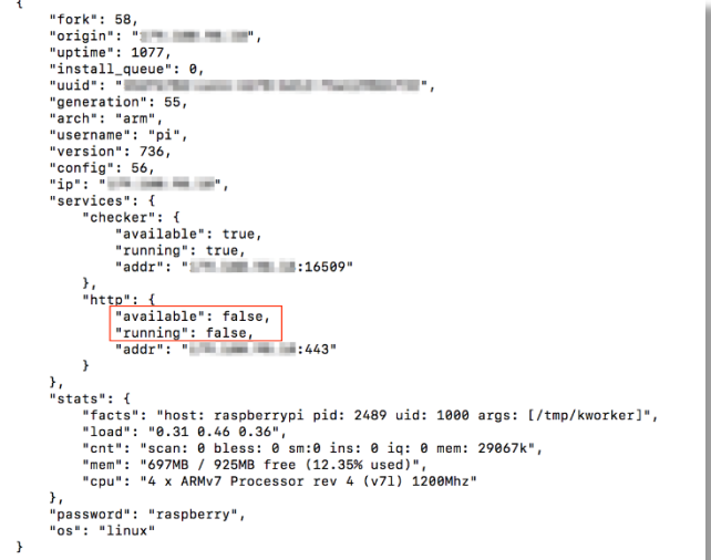
Figure 21. There are parameters under the section “http” indicating its IP address, “running” and “available” states.
